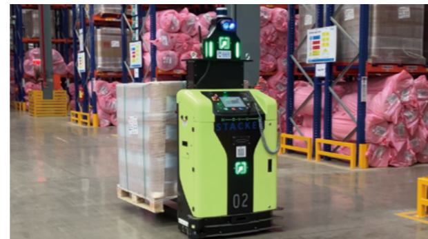
Inside the Mumbai Warehouse (During Operation of Auto Battery Operated Pallet Truck)
